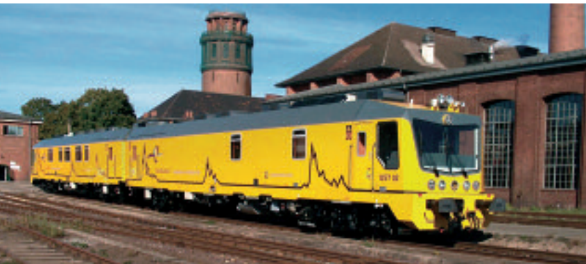
1 Rail Examination Train UST 02
